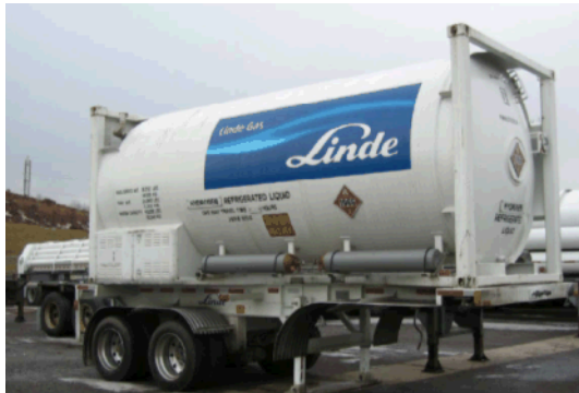
LH 2 Storage Tank
