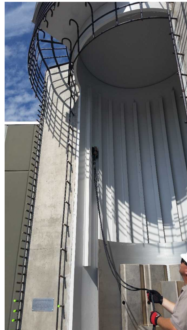
Testing a magnetic robot on a storage system cutaway, Palo Verde Nuclear Plant Education Center
