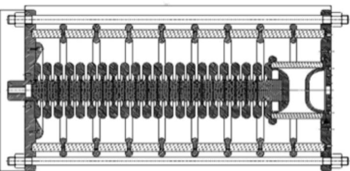
5.0-MV, 0.5-MA Laser-triggered gas switch
