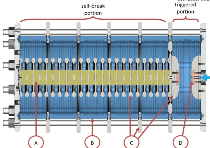
6.1-MV, 0.79-MA Laser-triggered gas switch
