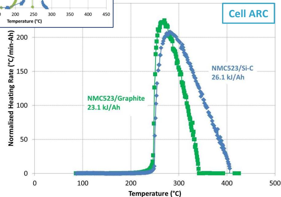
Thermal runaway enthalpy of NMC/Si-C cells is ~10% greater than NMC/Graphite cells
