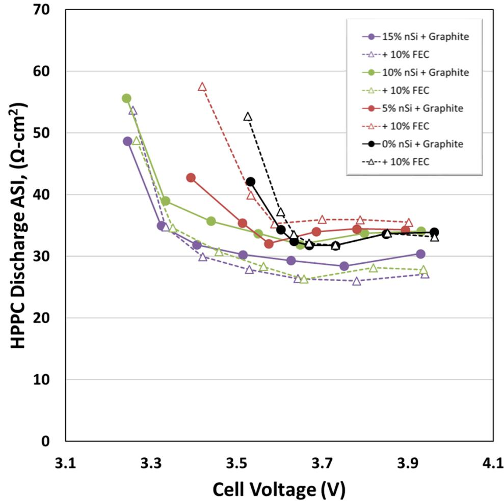
Lower nSi content electrodes demonstrate elevated ASI, reflecting issues experienced during coating process
