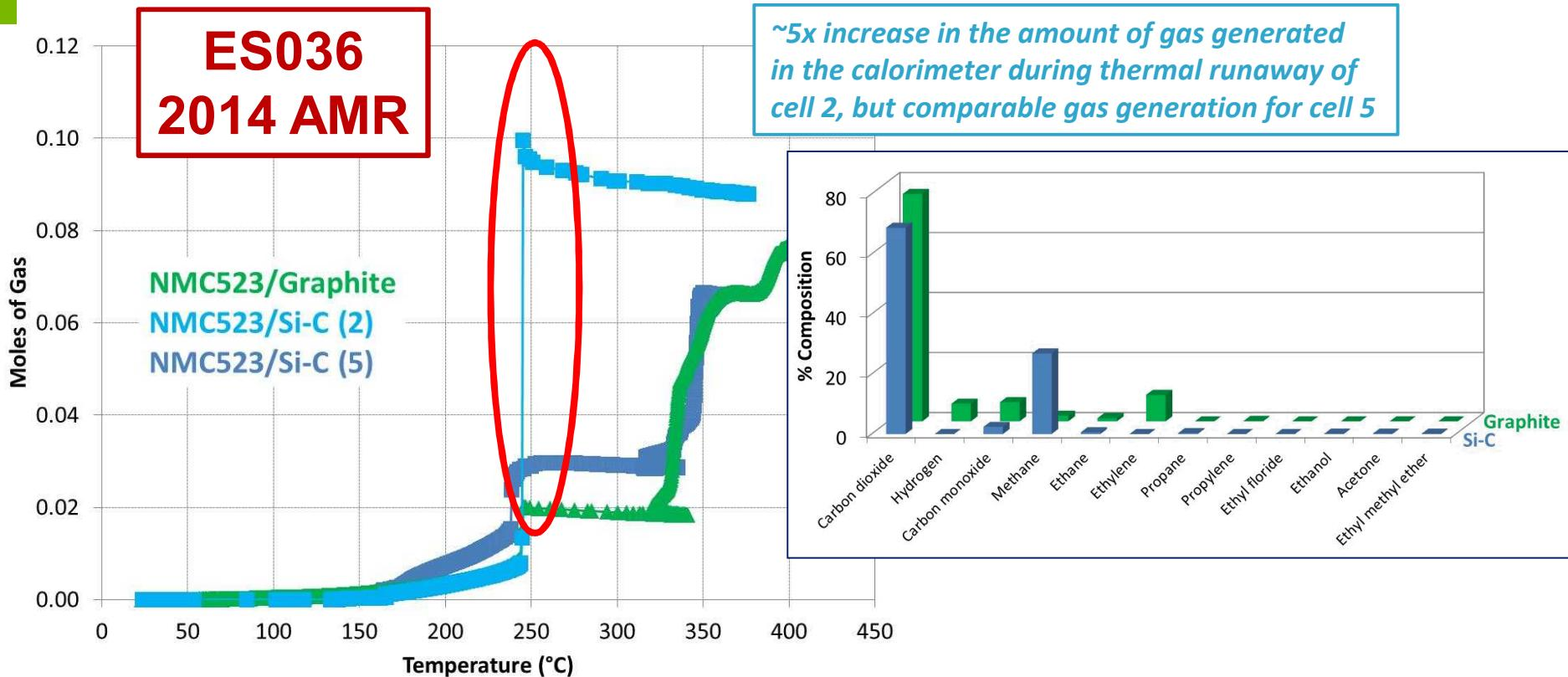
*Difference in gas generation attributed to the differences in surface reactivity and surface products generated at the anode/electrolyte interface*
