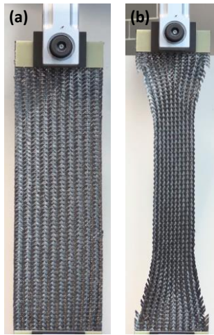
Figure 1. (a) 127 mm wide Twill Fabric at the start of the Bias Tension Test. (b) The same Twill Fabric following 100 mm extension.
