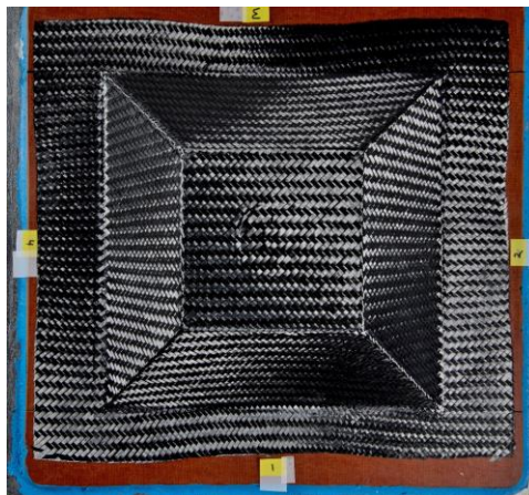
Figure 8. Top down view of twill fabric deformed from the \pm 45^\circ global orientation.
