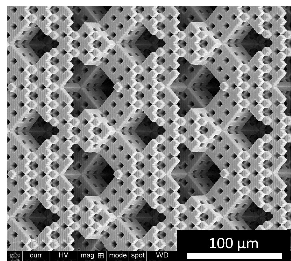
Above: Nanoscribe-printed 0.5-mm cube with  $40\text{ }\mu\text{m}$  lattice pores and  $8\text{ }\mu\text{m}$  sublattice pores. Right: cm-scale Ember-printed part with  $100\text{ }\mu\text{m}$  pores. Far right: Ember-printed part with  $250\text{ }\mu\text{m}$  lattice pores and mostly occluded  $50\text{ }\mu\text{m}$  sublattice pores, coated with a layer of palladium a few hundred nm thick by an aqueous chemical reduction technique.
