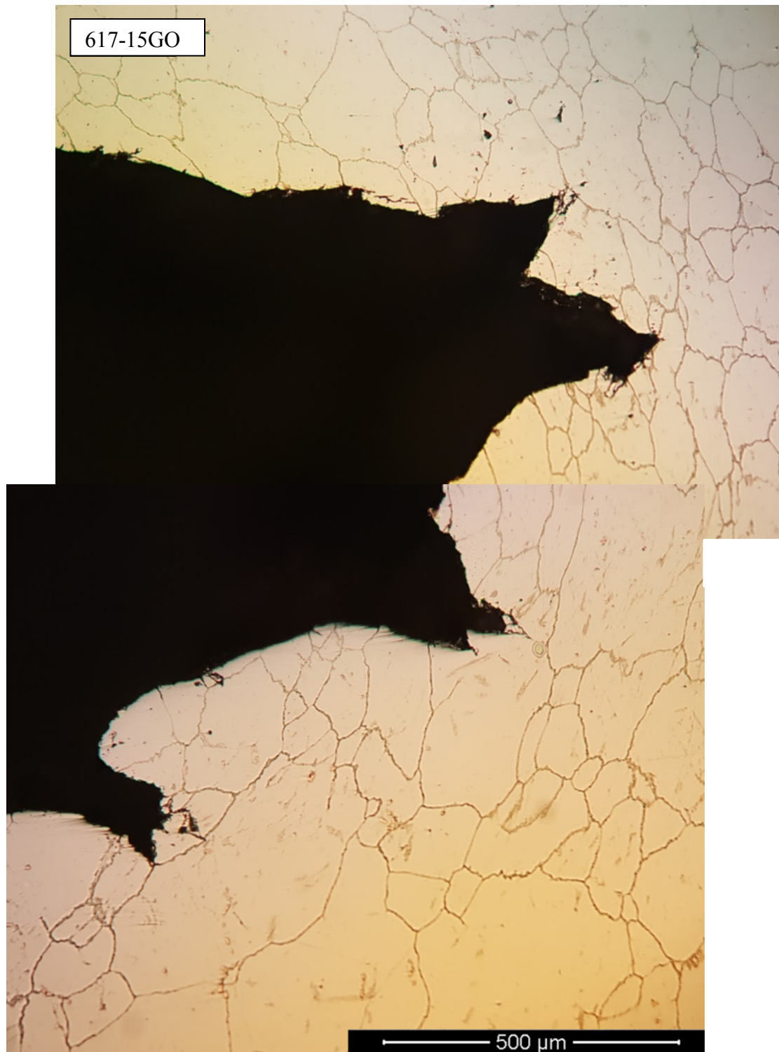
Fig. 47. 20x optical micrograph of etched profile of 617-15GO tested at 0.33 Hz with final \Delta K = 24.9 MPa \sqrt{\text{m}} .
