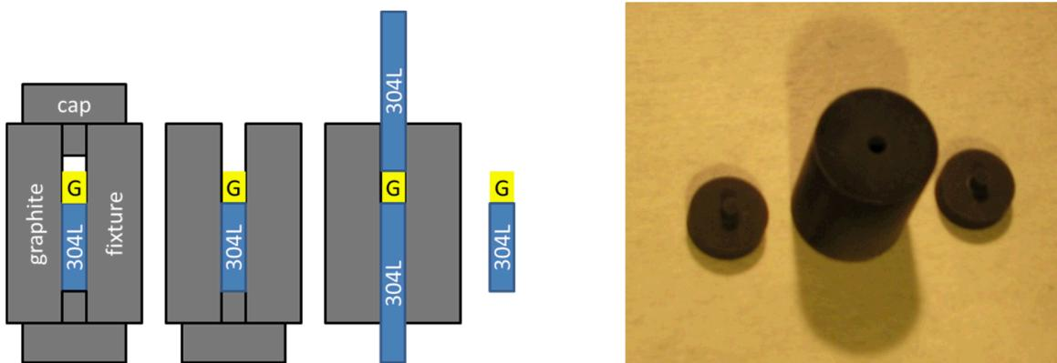
Figure 4. Graphite fixture for pin test and GC-pin configurations.
