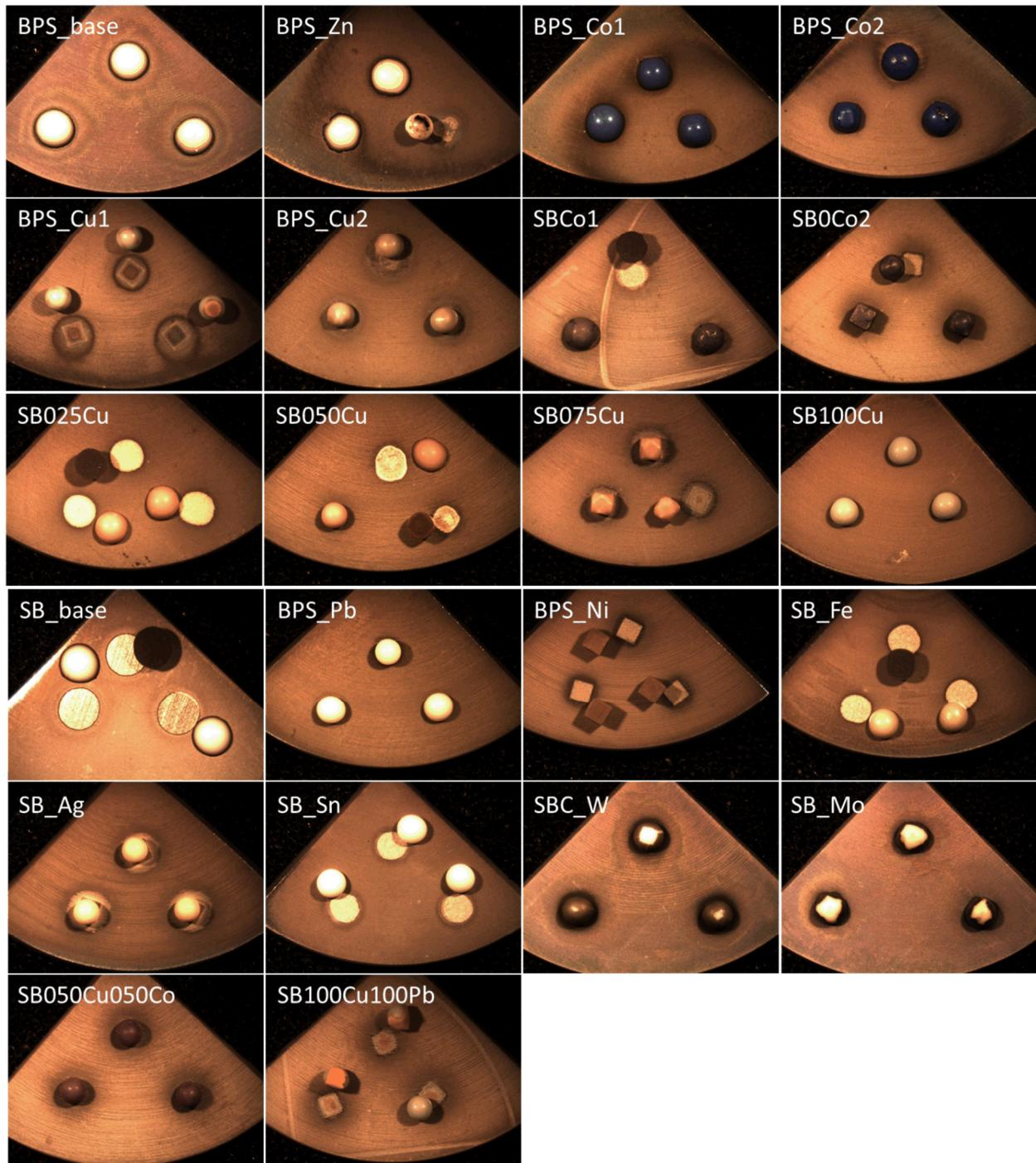
Figure 8. Sessile drop of all glass-ceramic specimens.
