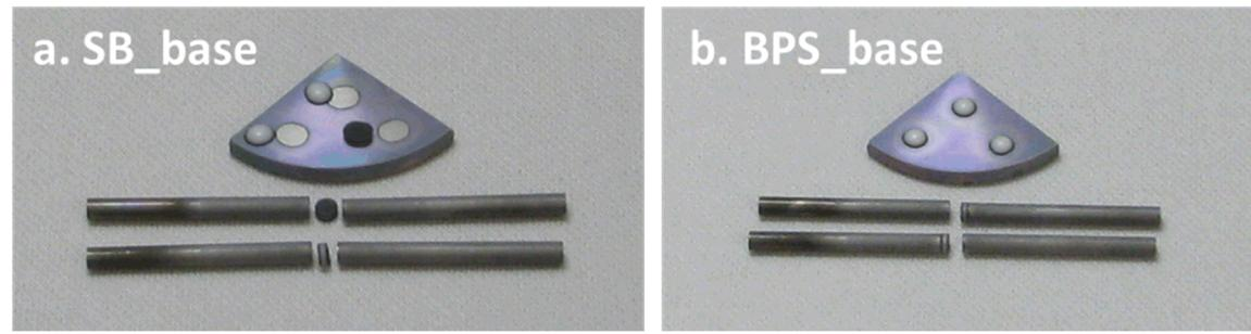
Fig 6. Images of (a) SB\_base and (b) BPS\_base glass-ceramics from sessile drop test open to furnace N<sub>2</sub> and pin bonding test in graphite fixture.
