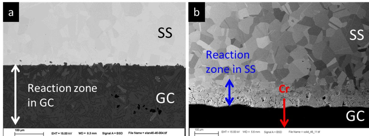
Figure 2. Amplified SEM view of, a) reaction zone in glass-ceramic with  $\text{Cr}_2\text{O}_3$  course  $\text{Li}_2\text{SiO}_3$  crystals, and b) EBS image showing the Cr depleted reaction zone in stainless steel.
