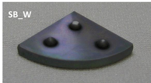
Fig 7. Discoloring of SB\_W glass-ceramic indicated  $\text{WO}_3$  being reduced at the surface.
