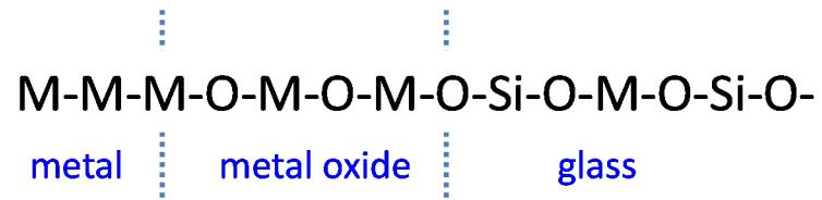
Figure 3. Schematic representation of chemical bonding between glass and metal.
