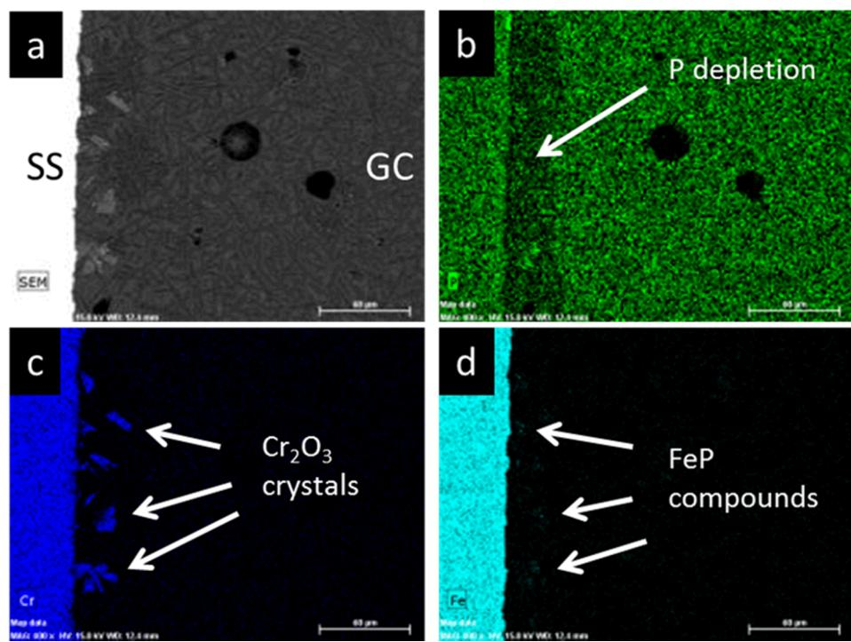
Figure 1. SEM cross section of GC-SS interface: (a) grey image, (b) P map, (c) Cr map, and (d) Fe map.
