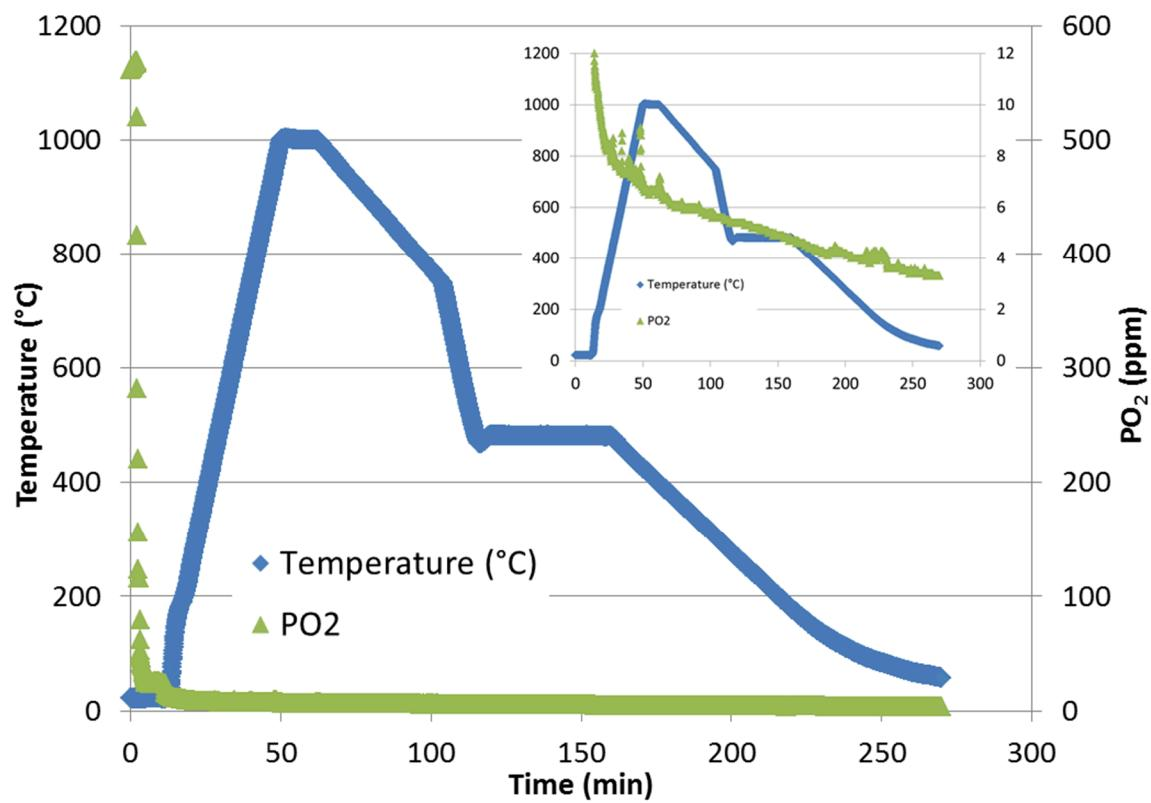
Figure 5. Oxygen partial pressure PO<sub>2</sub> in a sealing cycle with N<sub>2</sub> as processing gas. The insert shows expanded view of PO<sub>2</sub>.
