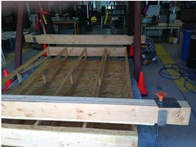
Figure 3 Testing of a rafter system. Image courtesy of Stephen Dwyer, Sandia National Laboratories
