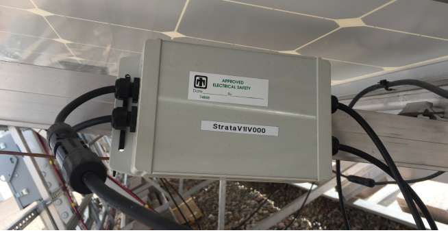
Fig. 1. Module level I-V curves where extracted from the module within the PV array using an in situ device. The device was controlled wirelessly and performed an I-V trace by extracting the module from the string. When it was finished it returned the module back into the string.
