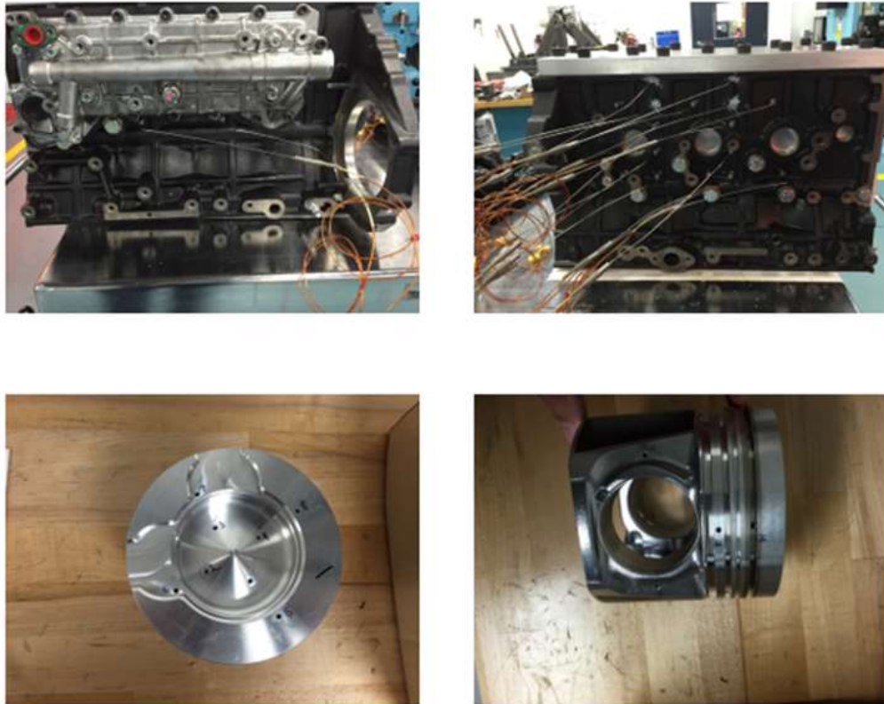
Figure 45 Instrumented block with thermocouples (top) and piston with templugs (bottom).
