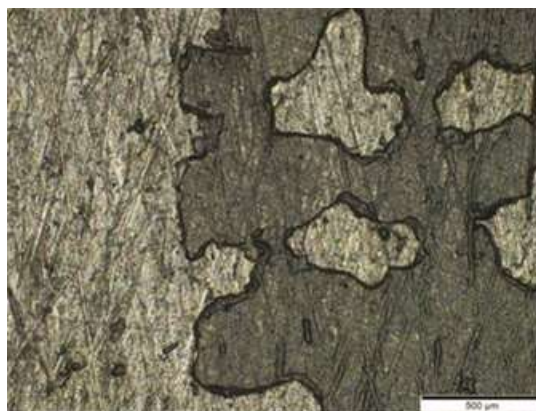
Figure 13 Micrograph showing coating delamination.
