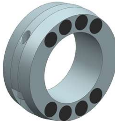
Figure 36 Bob weight to simulate the missing rotating/reciprocating mass.
