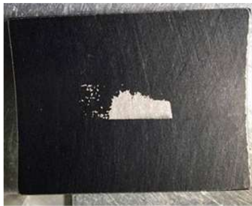
Figure 12 A cast-iron liner segment coated with a DLC coating from C2D showing delamination.
