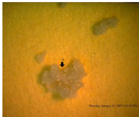
Figure 1. Digital Micrograph of Sulfuric Acid-filled Microcapsules on top of pH Paper before Mechanical Rupture
