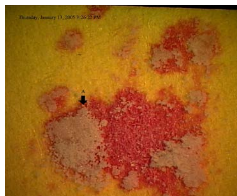
Figure 2. Digital Micrograph of Sulfuric Acid-filled Microcapsules on top of pH Paper after Mechanical Rupture
