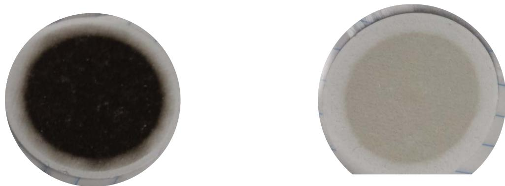
**Figure 111 Comparison of appearance of filters in steady state. Left = 30% output, Right = full output**
