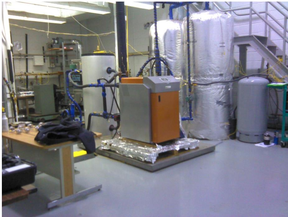
**Figure 3 Photo of 25 kW pellet boiler as tested and 119 gallon storage tank**
