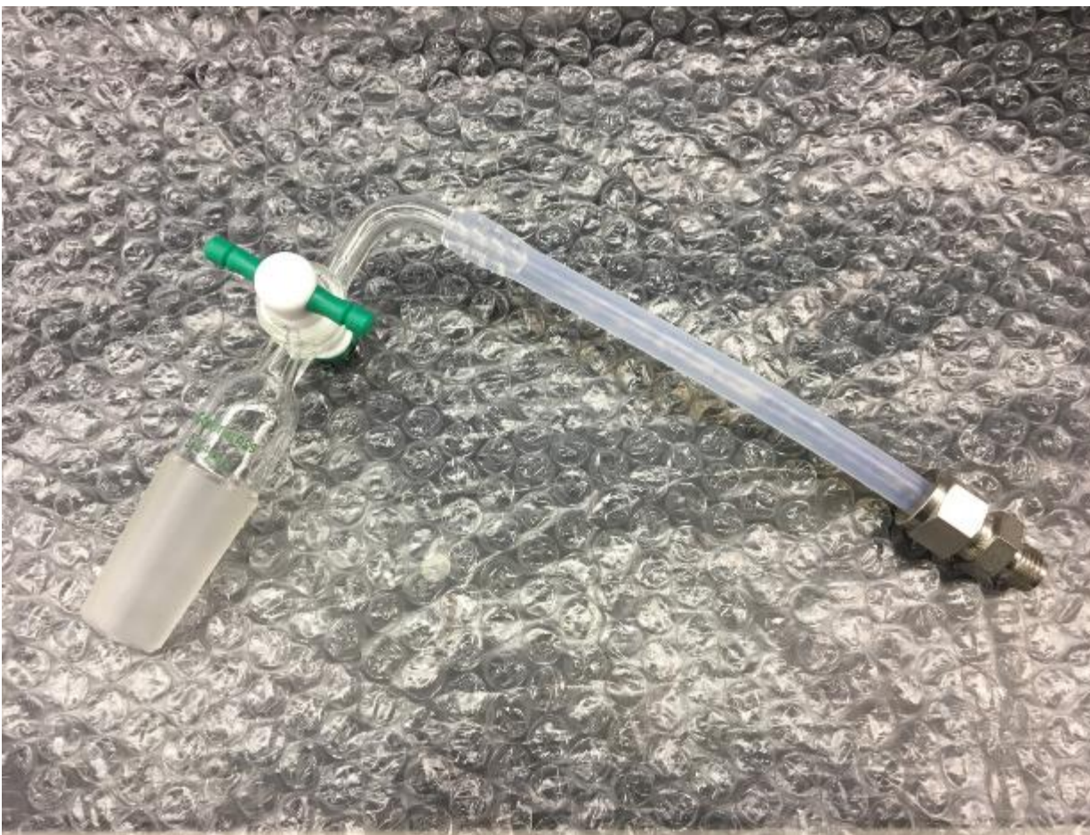
Figure 77: A reliable hermetic seal between a borosilicate glassware hose barb and slightly undersized thick-walled PTFE tubing (e.g. 3/8" OD, 1/4" ID) suitable for NO 2 service can be formed by preheating both the tubing and the hose barb and forcing the tubing over the hose barb.
