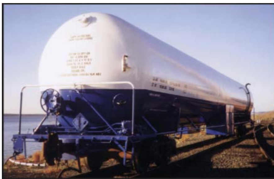
Figure 50: Cryogenic tank car used to carry liquefied natural gas (LNG) at a temperature of -162\text{ }^\circ\text{C} .
