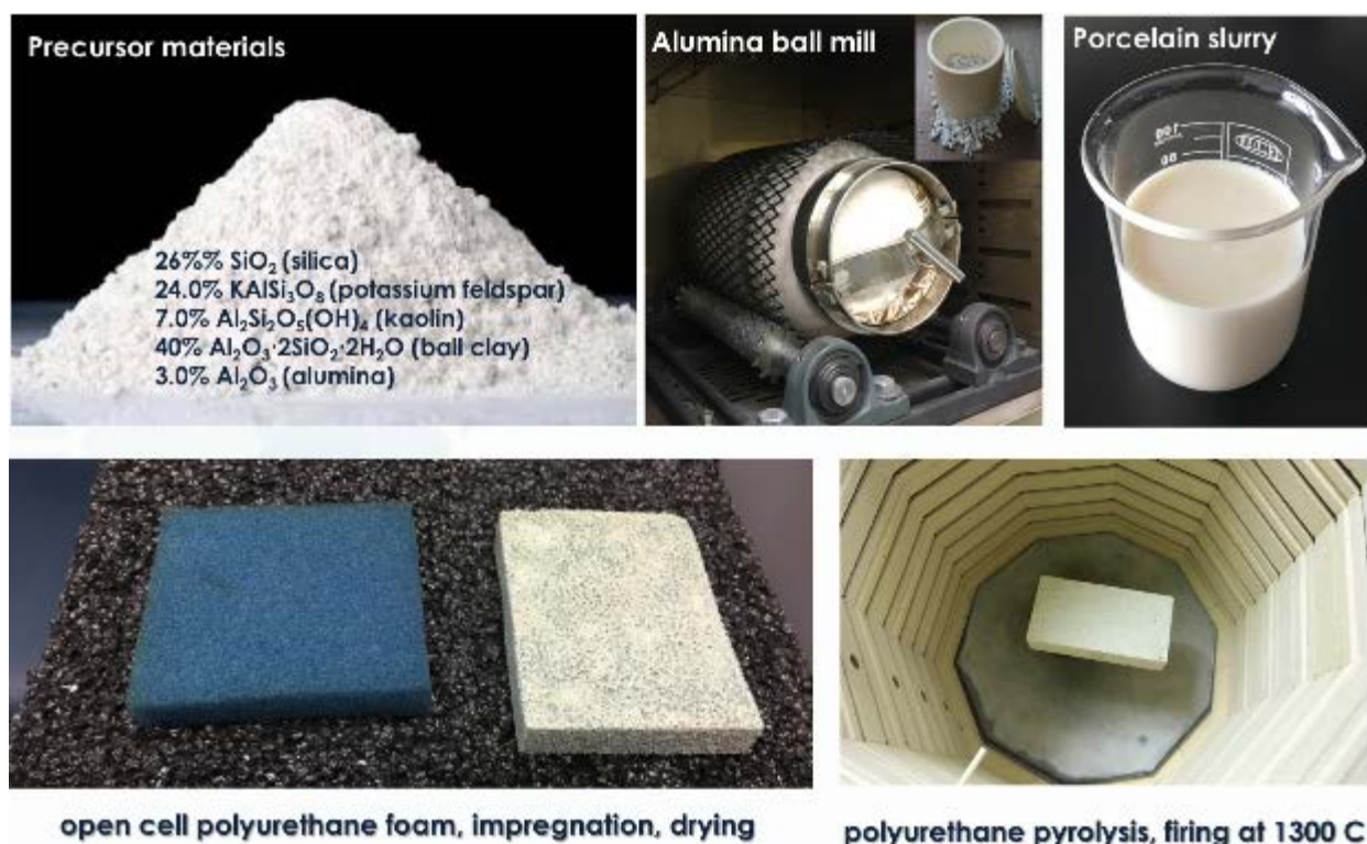
Figure 88: Fabrication of open-cell porcelain foam electrode cores.
