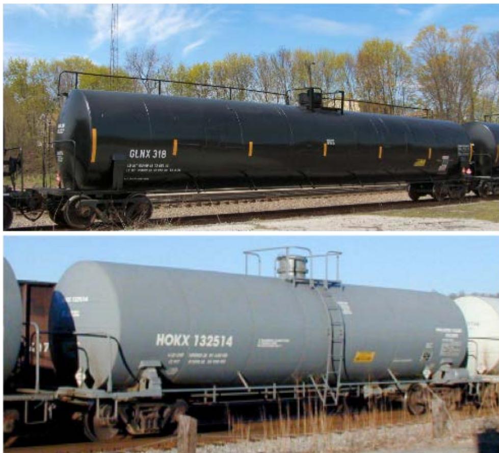
Figure 45: Top: DOT 105J300W tank car used for transport of molten sodium. Nameplate capacity = 33,600 gallons. Required outage for transport of molten sodium: 5%. Bottom: DOT 105A500W tank car used for transport of liquefied nitrogen dioxide. Nameplate capacity = 20,500 gallons. Required outage = 2%.
