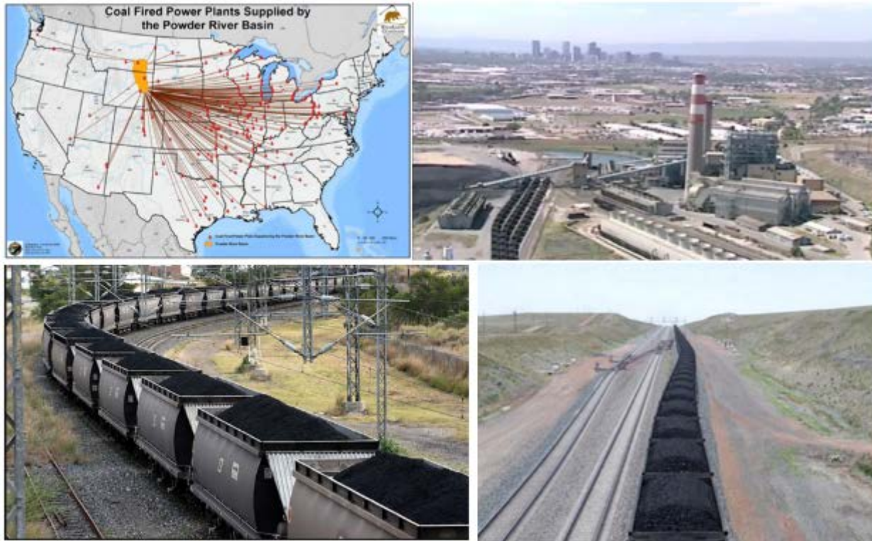
Figure 44: Much of the coal mined in the U.S. is transported several hundred miles by rail to coal fired electrical power generation plants located on the outskirts of population centers. Powder River Basin graphic from http://thinkprogress.org/climate/2011/03/26/207755/why-are-obama-and-salazar-pushing-a-massive-expansion-of-coal-mining/
