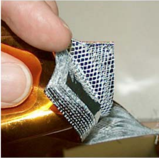
Figure 51: At left, multilayer insulation (MLI) construction showing metal coated plastic layers and scrim separator. https://en.wikipedia.org/wiki/Multilayer_insulation#/media/File:MultiLayerInsulationCloseup.jpg Original photo by John Rossie of AerospaceEd.org. At right, optimization of layer density to minimize combined heat transfer via conduction and radiation. See for example R. Barron, Cryogenic Systems , Oxford University Press, (1985).
