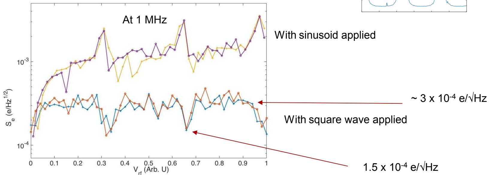
Usefulness as a charge sensor doesn't degrade as large signals ( $V_{rf}$ ) are used!
