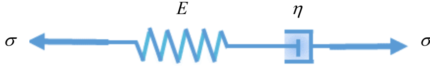
Figure 17. Maxwell model composed of spring in series with dashpot.
