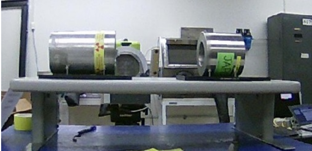
Figure 4. This optical image shows the 18-kg DU casting on the left and the 9-kg DU casting on the right. The spacing between the DU castings is 25 cm.
