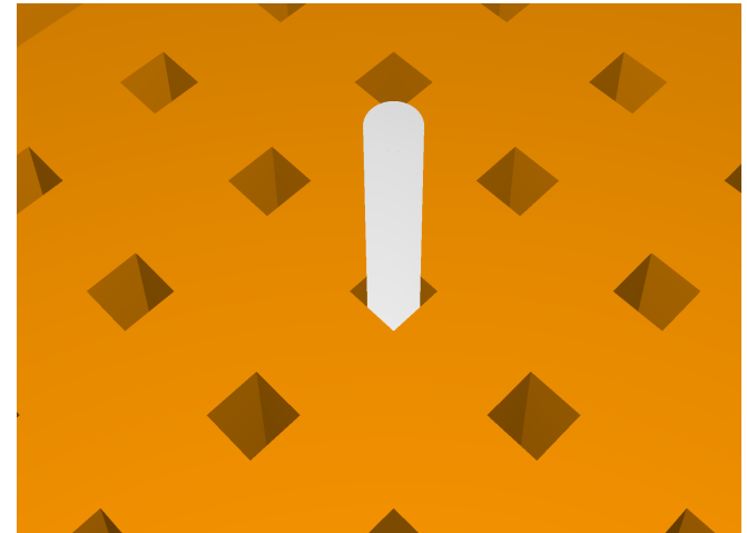
Detail view of CSG representation of a single rod in the pin assembly.
