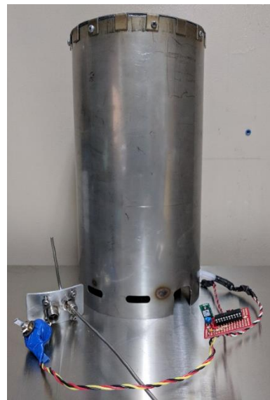
Figure 17. The P1 prototype was a standalone fan-powered unit. It was used to develop pressure curves that relate flow rate to fan speed.
