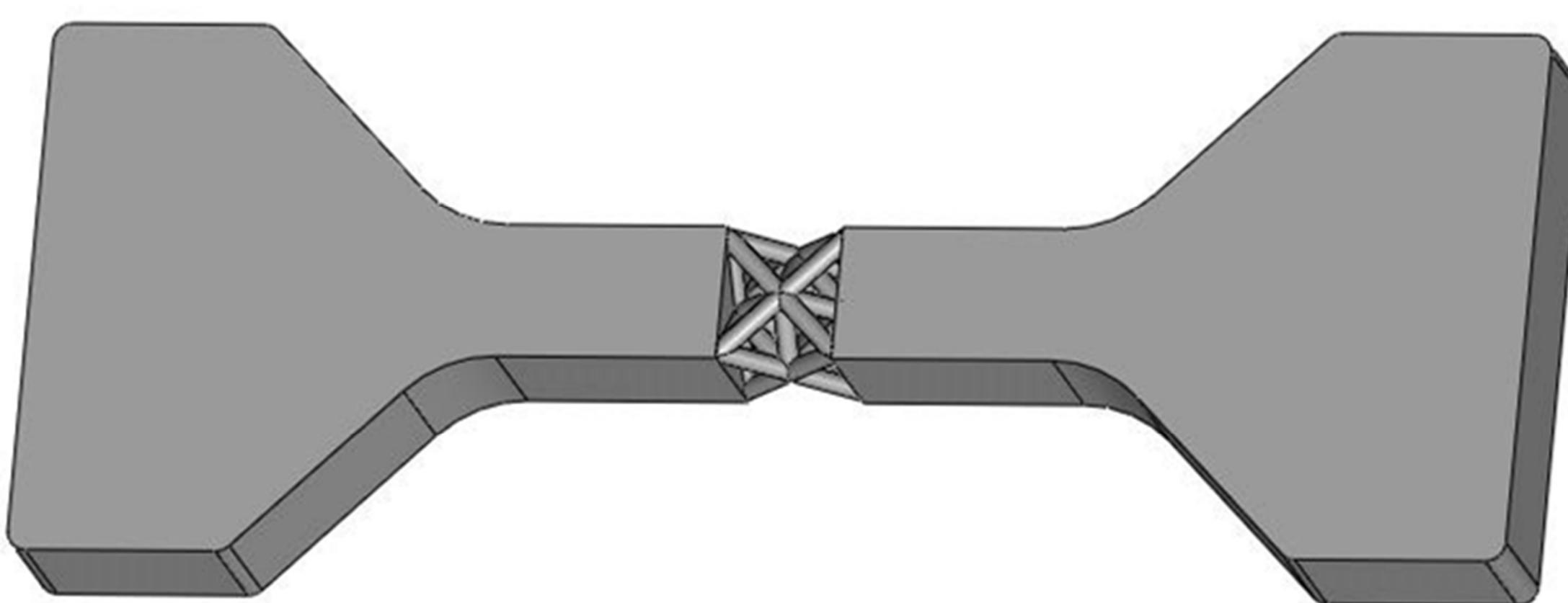
To achieve lattice properties, seven unit cells are joined in each direction within the gage section of the tensile bar, below.
