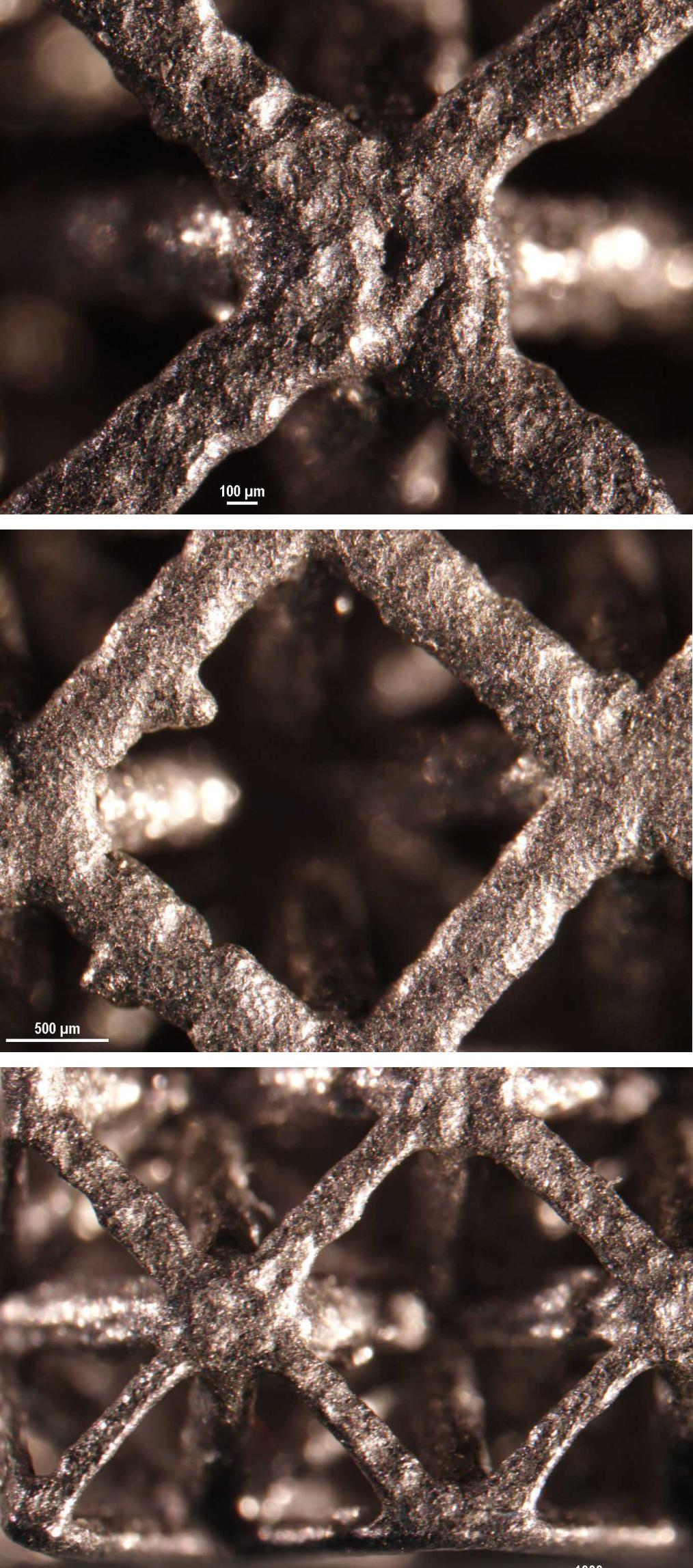
Two types of tensile bars will be built for these experiments. One bar will have a single unit cell in the gage section while the other has a 7x7x7 unit cell lattice. All tensile bars will be manufactured at Stratasys Direct Manufacturing in 17-4 PH stainless with stress relief and HIP treatment.
