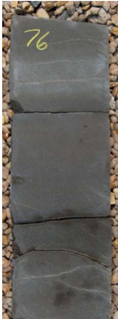
Macrofractures (induced & natural) visible in Middle Bakken core
