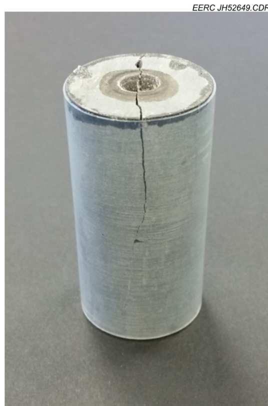
Figure 8. Sample 116219 posttest with injector removed.
