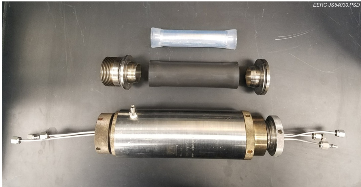
Figure 48. Inner gasket assembly and Hassler-style core holder.
