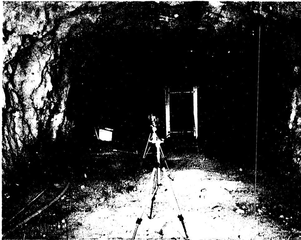
Figure 4.1-5. Prototype drift-mapping equipment in the G-Tunnel.
