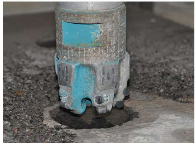
Figure 5. Photograph of the Ultrera 5-bladed PDC bit used in drilling tests.
