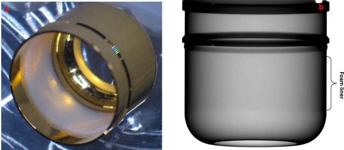
Figure 5: a) Optical image of a machined foam lined Au hohlraum half after cryogenic cycling. In this case, the nominal inner diameter of the hohlraum was 5.4mm and length was 5.06mm. Thickness of the 90mg/cc foam liner was 200 \mu m and its length was 2.5mm. b) X-ray transmission image where the high opacity of tantala makes the liner faintly visible through the 30 \mu m of Au wall of the hohlraum, a technique that offers a means of verification of the liner.
