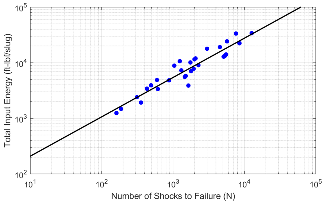
Figure 41. Plot of Number of Shocks to Failure versus Total Input Energy from SDOF Cantilever Beam Tests in CDL
