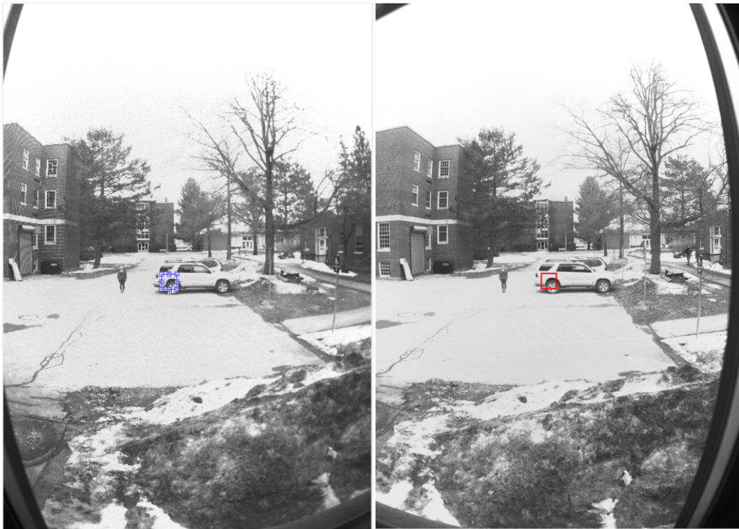
Figure 41. Normalized cross-correlation was used to successfully match the rear tire of a vehicle across a pair of images captured by the camera system. The template used is the area selected in blue on the left image, and the red region in the right image depicts the resulting match.
