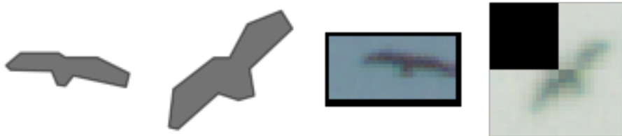
Figure 44. Simplified shapes with error of 4.25%, along with camera system images that the shapes were based upon.
