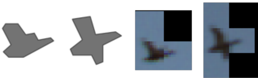
Figure 47. Simplified shapes with error of 8.5%, along with camera system images that the shapes were based upon.
