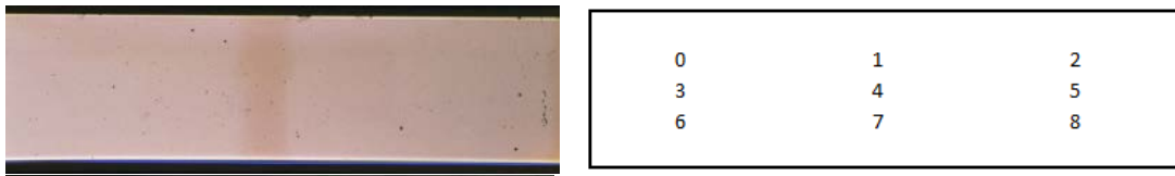
Figure 11. Left: white OLED in collaboration with OLEDWorks, 8.75" by 1.875" using our integrated substrate. Right: testing spots for brightness uniformity.
