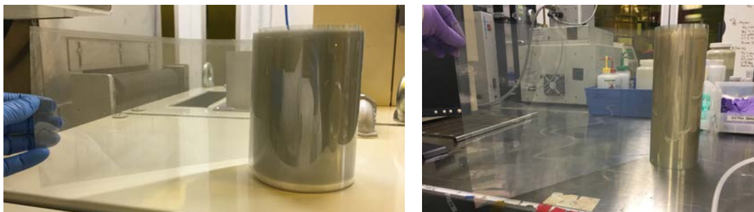
Figure 8. Photographs of 5"-wide and 12"-wide integrated substrates fabricated using only roll-to-roll methods.
