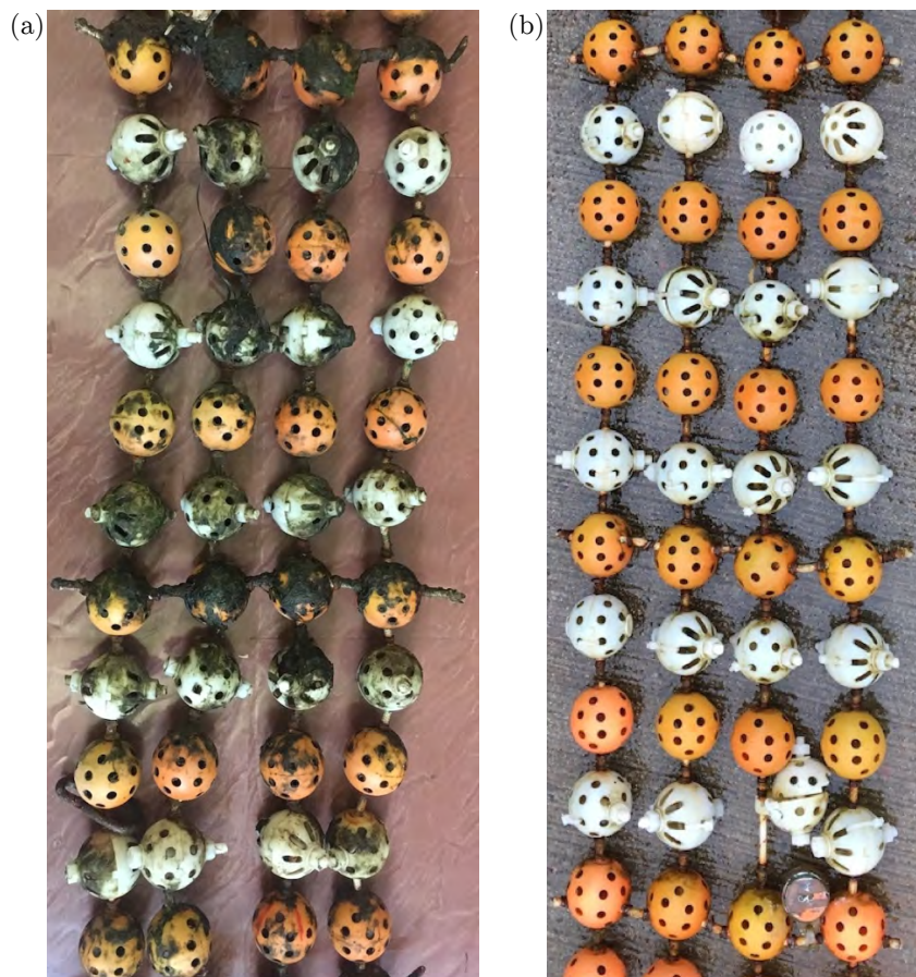
Figure 11.15: Biofouling on the (a) stationary net and (b) continuously moving net at the end of the ocean test.
