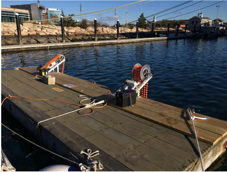
Figure 11.5: Both prototypes mounted to the wooden float and moored to the end of the MMA dock during testing.
