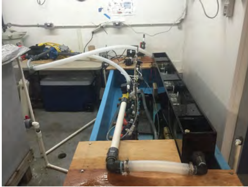
Figure 9.5: Flume tank setup with flow meter, centrifugal pump, and globe valve connected.
