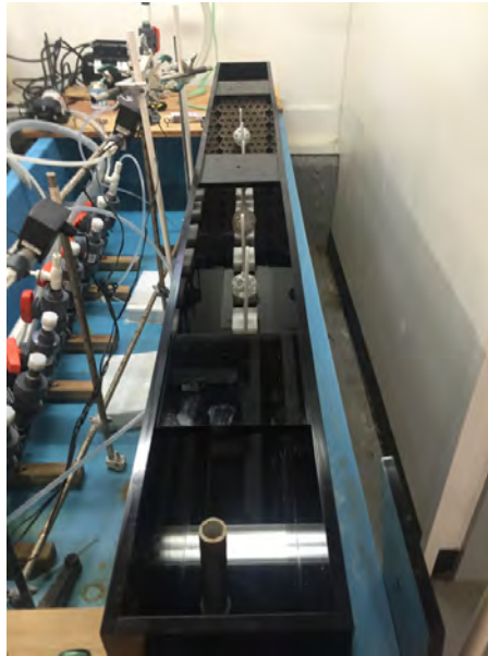
Figure 9.6: All six shells positioned in the flume tank.
