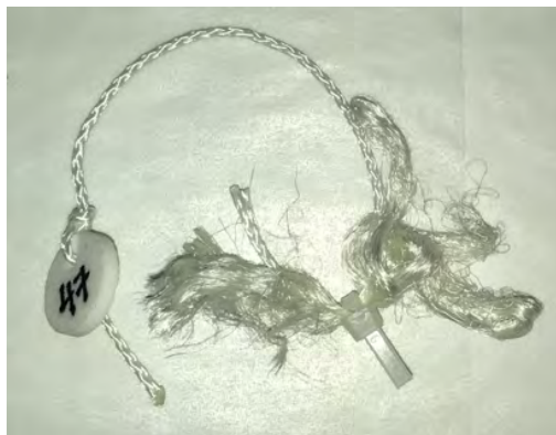
Figure 11.8: Pre-weighed adsorbent mini braid. One to two of these mini braids were placed in each shell design on each of the two prototypes.
