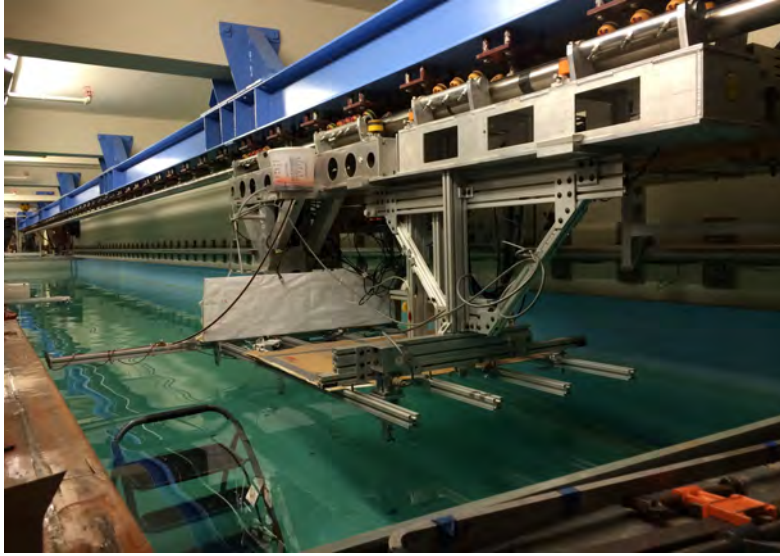
Figure 12.3: MIT Tow Tank where scale model hydrodynamic response tests were conducted of two designs of SMORE and the reference floating wind turbine.
