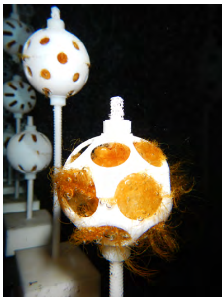
Figure 9.8: Photography showing the adsorbent in shells in the flume.
