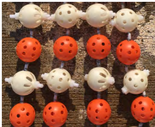
Figure 11.7: Small section of net with white shells for adsorbent fibers. Adsorbent enclosure shells were alternated with orange placeholder shells used for mechanical testing.
