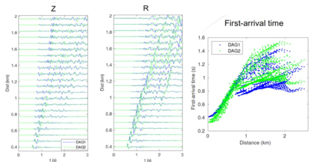
Result of purely seismic modeling (SPECFEM3D) in a 3D model of the second site of SPE, called DAG. Left: vertical and radial component along a SW-NE profile. Right: arrival time.
