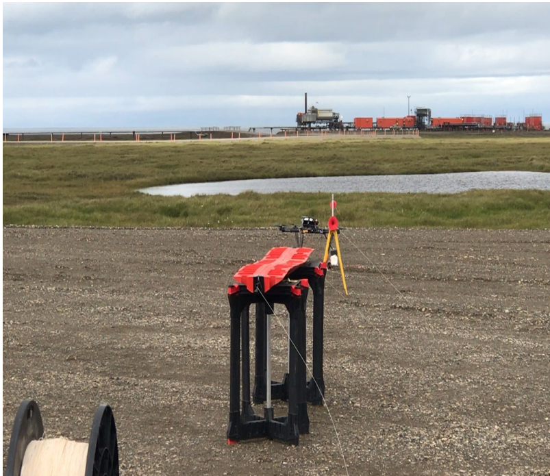
Figure 2. UAS preparing to ascend with fiber guide and heat tray shown between the UAS and motorized fiber spool.
