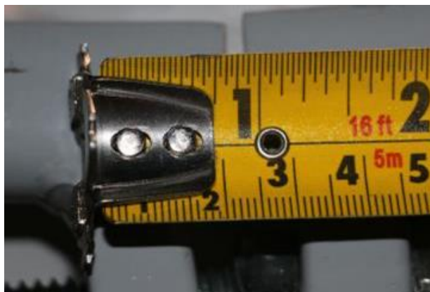
Figure 12. Gap that remains in the drum ring after torquing to 60 ft-lb. Image taken from the first test in
