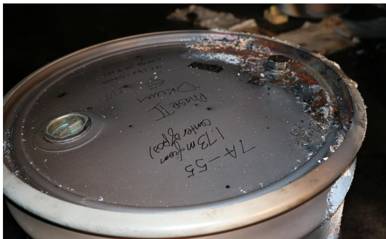
Figure 70. Conditions of the POC and 7As after completion of Test #2 in Phase II: (a) extent of damage to the center drum, (b) PC filter recovered from the center POC, and (c) and (d) damage on the lid of the POC and 7A drums closest to the fire.
