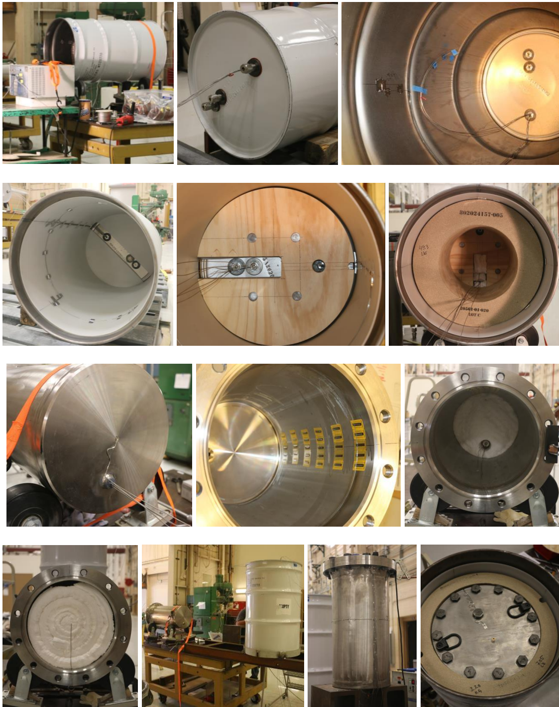
Figure 9. Series of images showing the process of instrumenting and assembling POCs in preparation for Phase I test. Images are from the first test.
