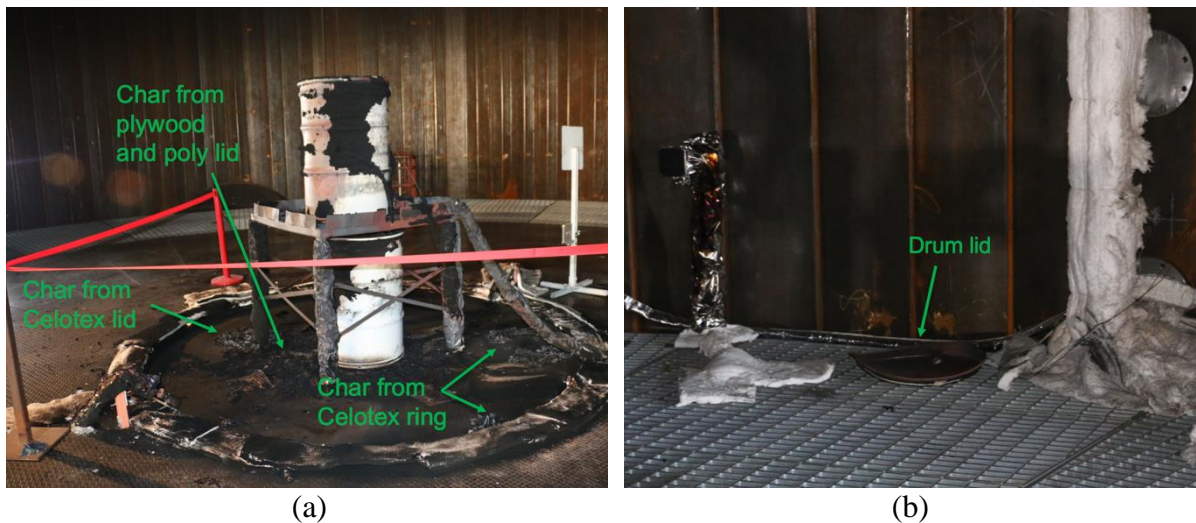
Figure 65. Test remains after Test #1 in Phase II. (a) center of the pool and (b) lid by the wall of the test cell.
