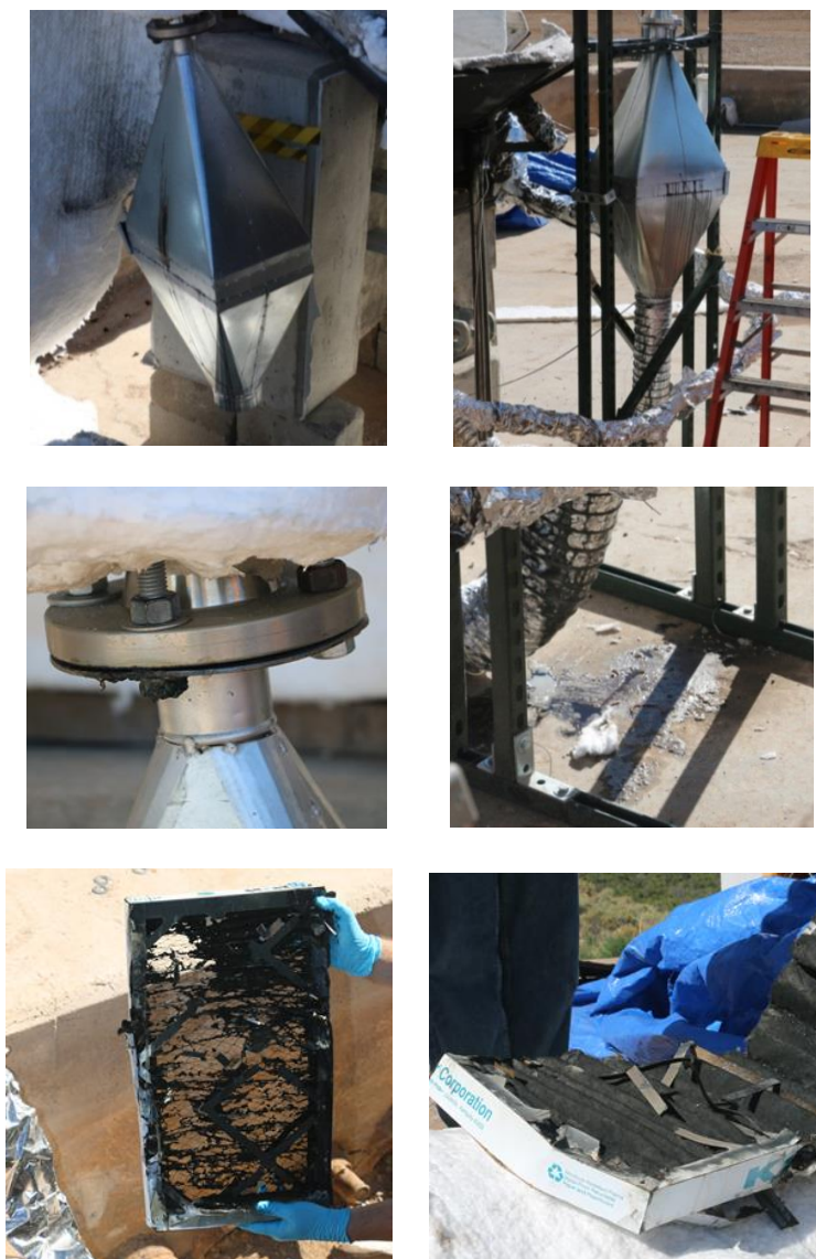
Figure 80. HEPA filter housing and HEPA filters after the test. Images shown on the left correspond to the air inlet side and on the right to the outlet air side.
