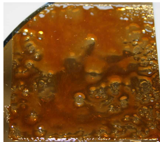
Bubbles: curing too high temperature without a step-cure profile (using syringe deposition method)
