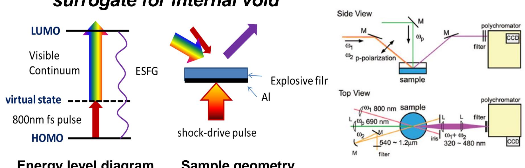
Schematic of electronic SFG experiment. Visible and IR pulses are combined at surface to probe electronic structure of interface. Sum frequency signal is emitted in unique spatial direction. Signal is produced by nonzero  $\chi^{(2)}$  susceptibility within few molecular layers of surface.
