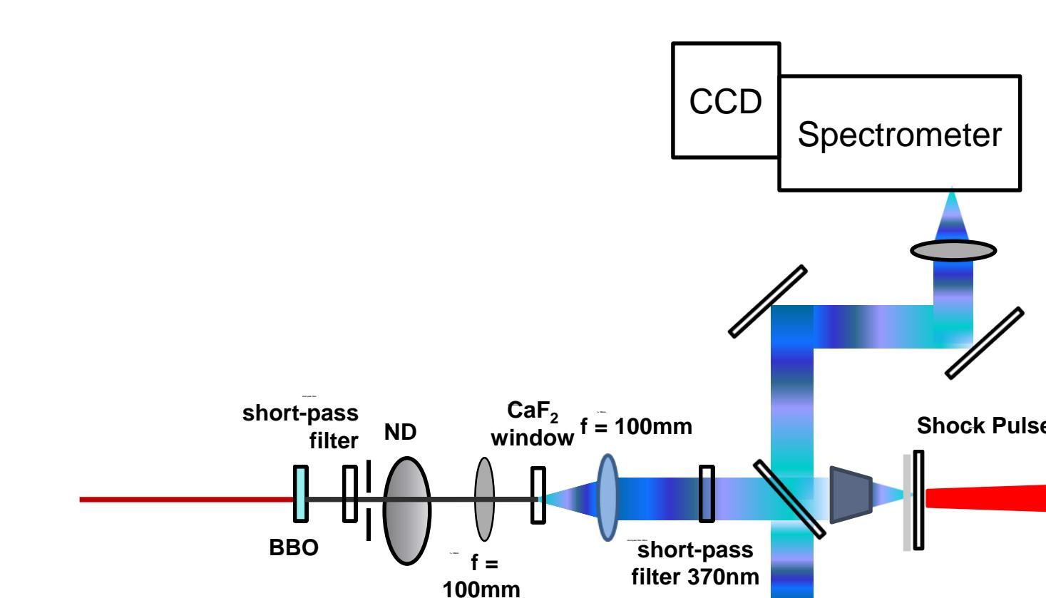
Schematic of transient absorption experiment. Broadband ultrafast pulse probes change in absorption spectrum of bulk during shock compression.
