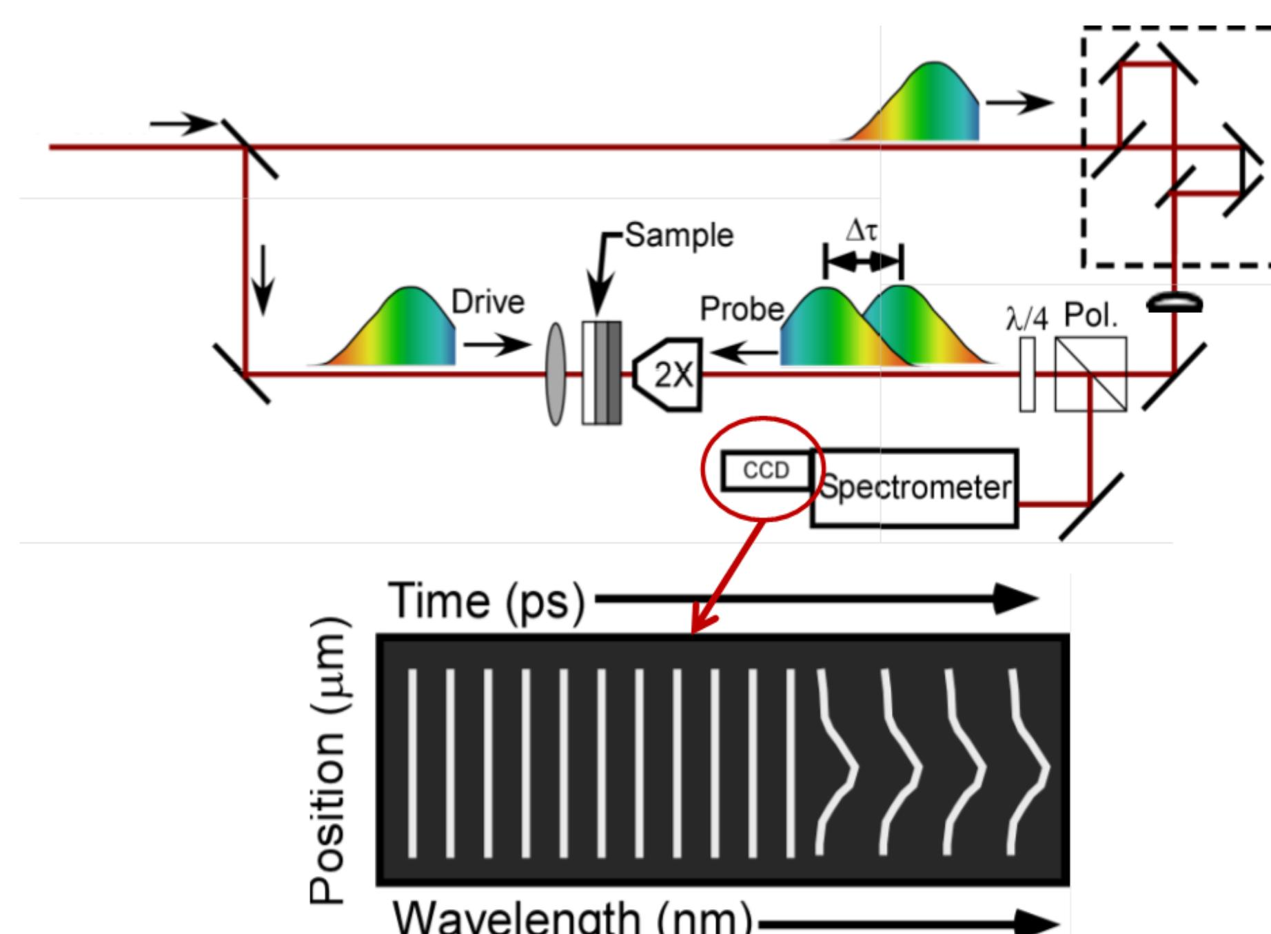
Schematic of USI setup. Technique developed at LLNL and implemented at Sandia for Shock Characterization
