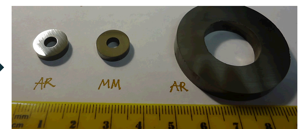
Net-shaped and sintered toroids (no machining required)
