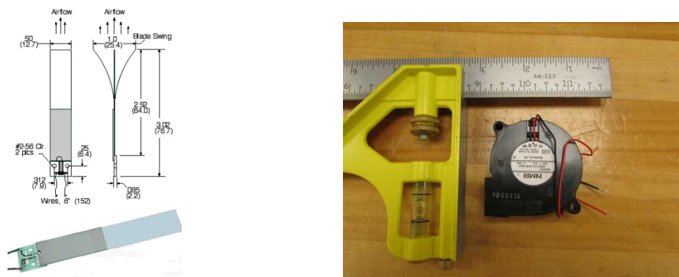
Figure 8: On the left is a schematic of a one blade piezoelectric fan. On the right is a picture of a mini DC blower.
