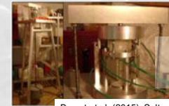
Dead weight setup Sample size: \varnothing=70 mm L = 140 mm
