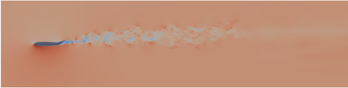
Figure 5: Zoomed slice through the wing of a PHASTA simulation.
