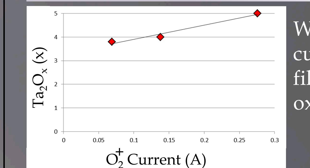
• Density, Resistivity & Stoichiometry are all correlated. As shown above, a slight current change in the ion gun can make a change that allows multiple film sub-stoichiometry states to be studied very easily.
