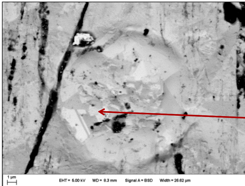
Backscattered electron channeling contrast image of Pd-Ag-Cu alloy after high current exposure
