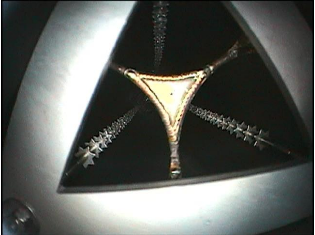
Figure 1.9. Photograph looking down into the WESP from the top. The three channels with electrodes are visible.
