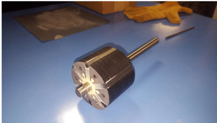
Figure 23: The second IPM rotor with production intent ferrite magnets
