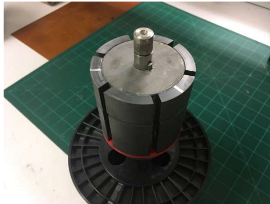
Figure 42: 6-pole surface mounted prototype rotor, with ferrite magnets
