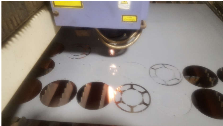
Figure 18: Stator laminations being laser cut in the QM Power shop
