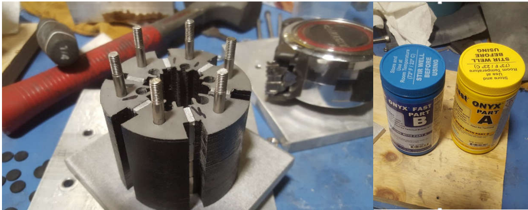
Figure 16: Rotor pole pieces assembled on a fixture with the magnets in preparation for casting the urethane hub; the motor shaft would also be inserted in the fixture prior to casting
