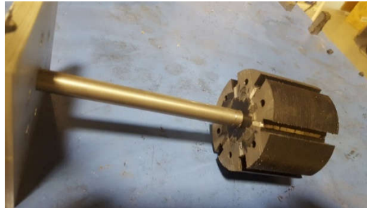
Figure 17: Prototype rotor assembly after curing of the urethane and removal from the fixture
