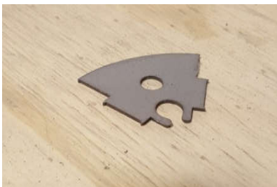
Figure 15: Laser cut individual rotor pole lamination for the NdFeB design
