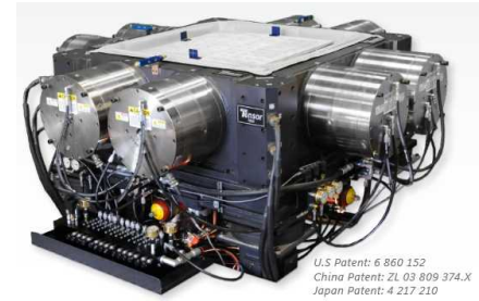
Fig. 2 Tensor 18kN multi-axis vibration test system [23]
