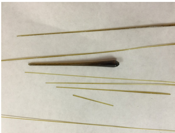
Figure 18. Optical image of \text{GeS}_2 fiber drawn and remnants of the preform.
