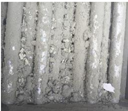
Figure 5. Photograph of accumulated material on the top section of the tube bundle from E-110
