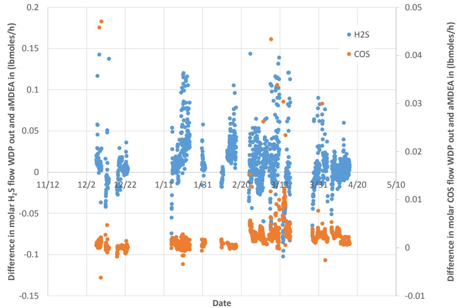
Figure 47. Differences in molar flows of sulfur species out of WDP and into aMDEA® for mass balance calculations
