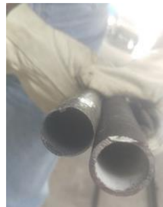
Figure 4. Sections of E-110 tube (the thinned tube on the left and normal tube on the right)
