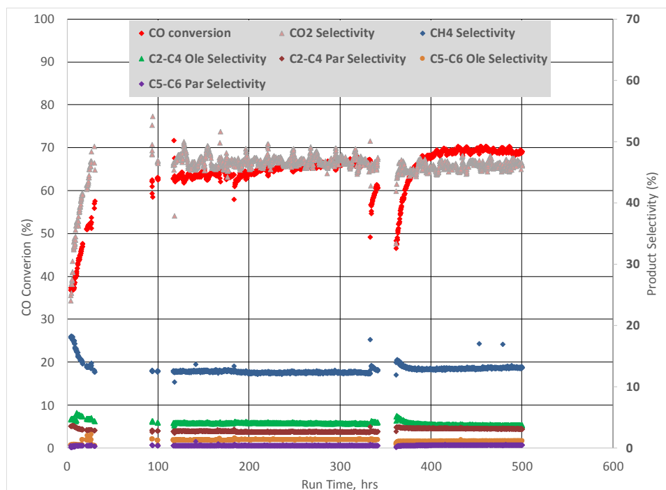
Figure 55. Fe-based FT catalyst CO conversion and product selectivity for baseline test
