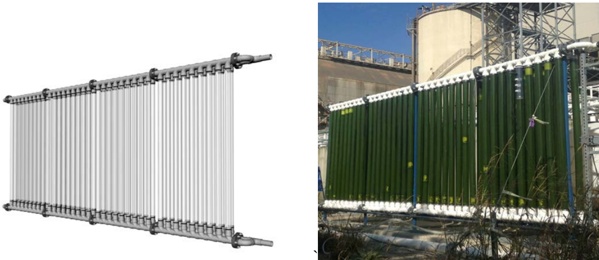
Figure 2. Overhead view of parallel manifolds showing alignment of tubes to minimize shading [18].
