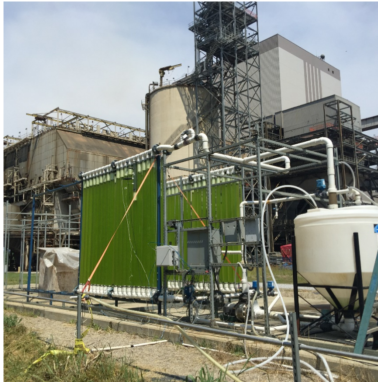
Figure 25. Cyclic flow reactor at initial culture density of 0.06 g/l
