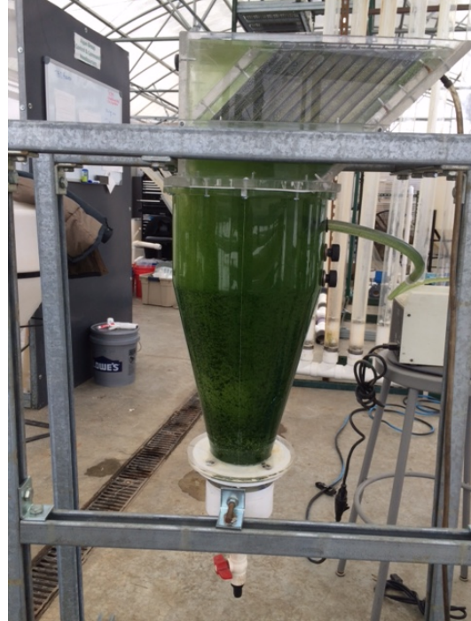
Figure 61. Lamella thickener after 2 hours of operation.
