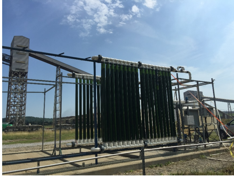
Figure 26. Cyclic flow reactor ready to be harvested (1.1 g/l culture density)
