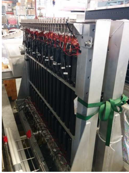
Figure 5. Trigger scintillators on loan from Tohoku University to be used in the Bethe-Heitler measurements at \text{HI}\gamma\text{S} . They were previously used at JLAB.
