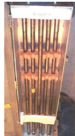
INTR tamper indicating items (fuel rods at left and right, welded container above).
