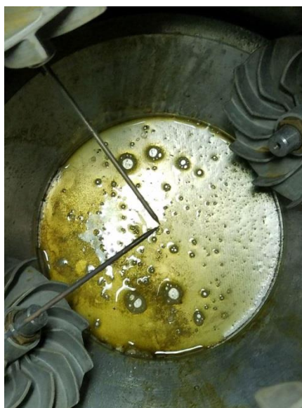
Fig. 108 Water condensed inside the bomb after 10 bar experiment. The oxidizer was air ( O_2:N_2:1.0:3.76 ). Hydrogen was burned at \phi=0.5 . Top view.
