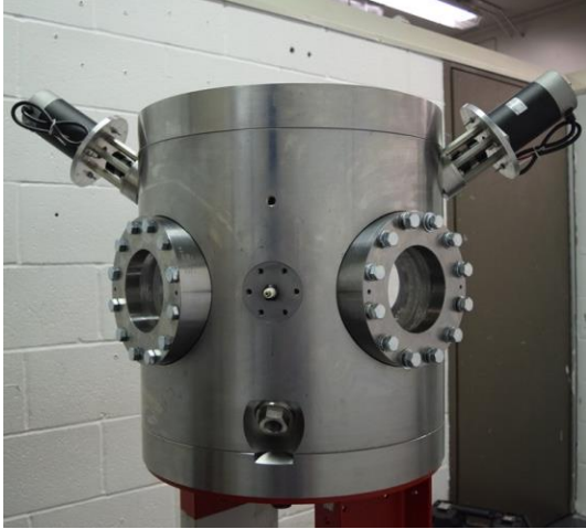
Fig. 82 Turbulent flame bomb during assembly. Plumbing and wiring work is missing in this picture.
