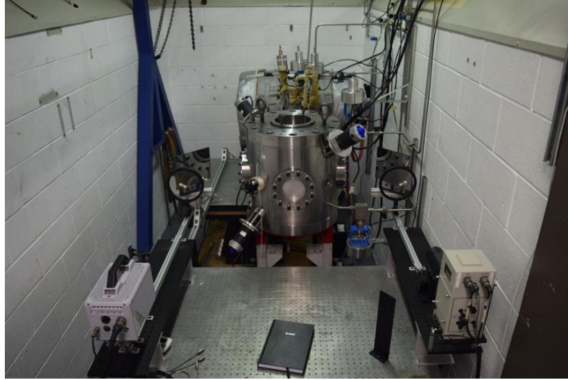
Fig. 113 Blast room layout. The new fan-stirred flame bomb is at center. An existing, heated, stainless steel, laminar flame vessel is partially visible in the back. The schlieren optical elements are shown.
