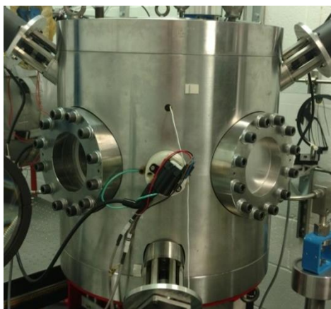
Fig. 105 The quartz substrate on the right window has been substituted by aluminum blank.
