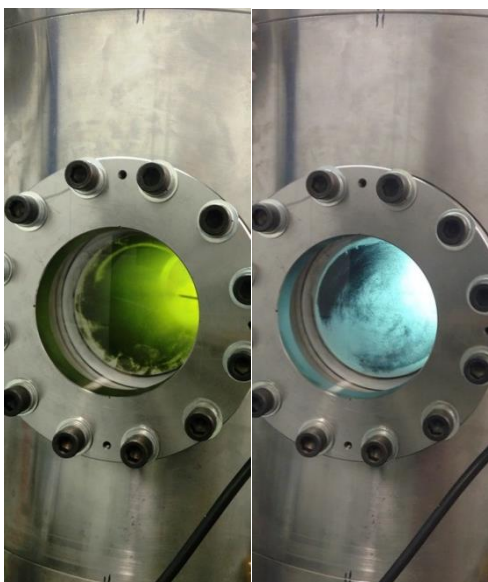
Fig. 107 Combustion products after a 10 bar experiment. The oxidizer for the left side was O_2:N_2::1.0:3.76 . The oxidizer for the right side was O_2:He::1:6 .
