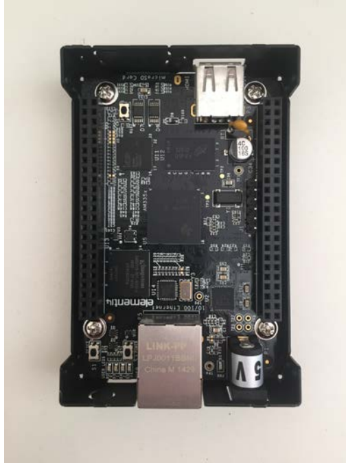
Figure 4. BeagleBone Black embedded Linux computer
