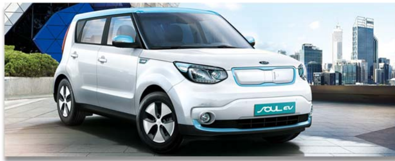
Figure 5: The 2015 Kia Soul EV was used as a surrogate vehicle with SAE J1772 standard compliance AC Level 1 and Level 2 charging as well as DC fast-charging CHAdeMO" (CHAdeMO) infrastructure.
