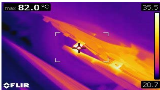
Figure 26: High heat affects left mounting bracket. A forward-looking infrared camera (FLIR) captured the heat signature of the receiver's left mounting bracket at 82C at 161 minutes of system charging.
